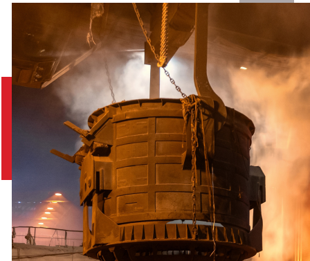
Argon stirring at ladle furnace
